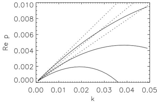
Fig. 14. Magnetic field growth rate  $\text{Re } p$  as a function of  $k$  for  $k$  small and  $R = 32, 64$  and  $128$  (reading down the solid curves). The dotted curves give the low- $k$  prediction from the  $\alpha$ -effect calculation.
