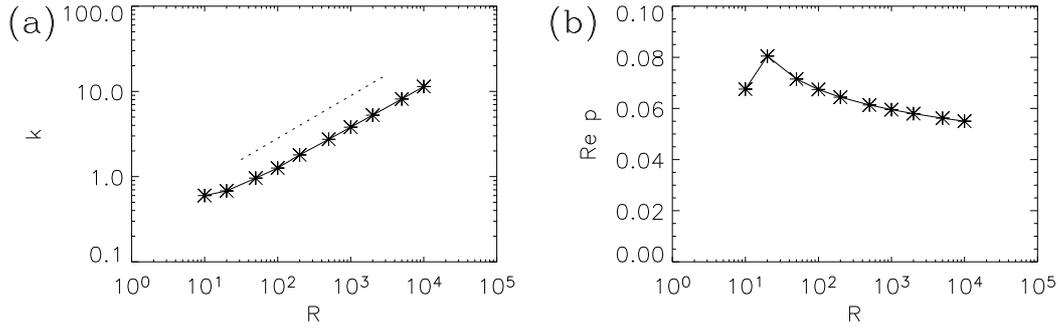
Fig. 11. In (a) the wave number  $k$  and (b) the growth rate  $\text{Re } p$  for the fastest growing cat's eye mode, are plotted against  $R$ . The dotted line in (a) shows the scaling  $k \propto R^{1/2}$ .
