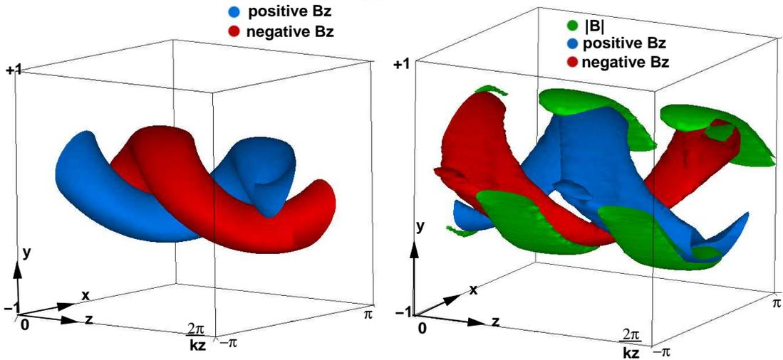
Fig. 4. Magnetic field as in figure 2 but with plots of isosurfaces,  $B_z = B_{z0}$  (blue),  $B_z = -B_{z0}$  (red) and, in (b) only,  $|\mathbf{B}| = B_0$  (green). In (a)  $k = 2.5$  and we have  $B_{z0} = 0.5 \max B_z$  (with  $\max B_z \simeq 0.6 \max |\mathbf{B}|$ ), and in (b)  $k = 5$  and the levels  $B_{z0} = 0.65 \max B_z$ ,  $B_0 = 0.65 \max |\mathbf{B}|$  are used (with  $\max B_z \simeq 0.1 \max |\mathbf{B}|$ ).
