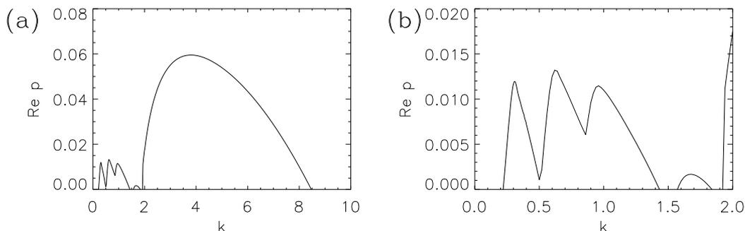
Fig. 8. Magnetic field growth rate  $\text{Re } p$  as a function of  $k$  for  $R = 1000$  and flow (3.2), (3.3); (b) is simply a magnified view of the bottom left corner of (a).
