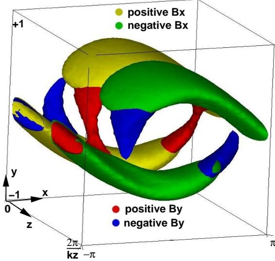
Fig. 5. Magnetic field as in figure 4(b) with  $k = 5$ , but with plots of isosurfaces,  $B_x = B_{x0}$  (yellow),  $B_x = -B_{x0}$  (green),  $B_y = B_{y0}$  (red), and  $B_y = -B_{y0}$  (blue). Here  $B_{x0} = 0.25 \max B_x$  and  $B_{y0} = 0.28 \max B_y$ , with  $B_{x0} \simeq \max |\mathbf{B}|$  and  $B_{y0} \simeq 0.25 \max |\mathbf{B}|$ .
