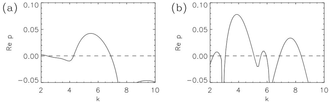
Fig. 12. Magnetic field growth rate  $\text{Re } p$  as a function of  $k$  for  $R = 1000$  and flow (3.7) with (a)  $\phi = \pi/36$  and (b)  $\phi = \pi/12$ .
