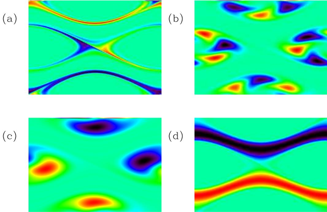
Fig. 9. Magnetic field structure for  $R = 1000$  and (a)  $k = 3.8$  (cat's eye mode), (b)  $k = 1.0$  (Ponomarenko mode,  $m = 3$ ), (c)  $k = 0.3$  (Ponomarenko mode,  $m = 1$ ), and (d)  $k = 0.001$  ( $\alpha$ -effect mode). In each case  $B_z$  is plotted in the  $(x, y)$ -plane with positive field yellow/red and negative field blue/black.
