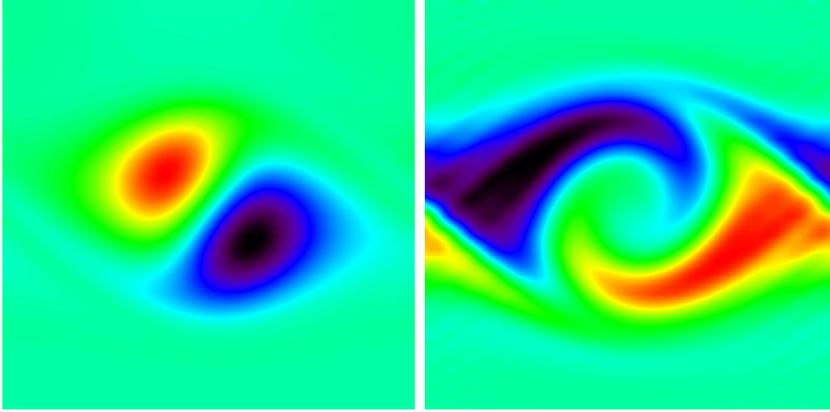
Fig. 2. Magnetic field in the flow (2.4) with  $R = 500$ . In (a) there is a Ponomarenko mode with  $k = 2.5$ , and (b) a cat's eye mode with  $k = 5$ . In each case  $B_z$  is plotted in the  $(x, y)$ -plane with positive field yellow/red and negative field blue/black.
