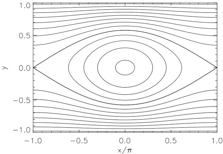
Fig. 1. Stream lines of constant  $\psi(x, y)$  are shown for the flow (2.4). The flow is periodic in the  $x$ -direction.
