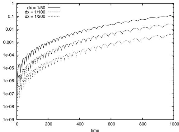
FIG. 9: The  $\Theta$  quantity is plotted for three different resolutions ( $dx = 1/50$ ,  $dx = 1/100$ ,  $dx = 1/200$ ) with the Q4 gauge and  $\eta = 1$ , showing a (second order) convergence to the exact zero solution.
