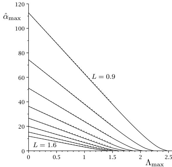
FIG. 6: Plot of the relationship between the critical inclination angle  $\hat{\alpha}_{\max}$  and the critical external airflow strength  $\Lambda_{\max}$  for  $L = 0.9, 1, 1.1, 1.2, 1.3, 1.4, 1.5, 1.6$ . The dotted lines show the first-order-accurate asymptotic solutions in the limit of a weak external airflow,  $\Lambda \rightarrow 0^+$ .
