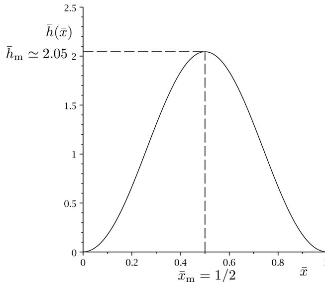
FIG. 9: Plot of the leading order scaled ridge profile  $\bar{h}(\bar{x})$  in the limit of a strong external airflow,  $\Lambda \rightarrow \infty$ , obtained by solving (31) subject to (32) numerically.
