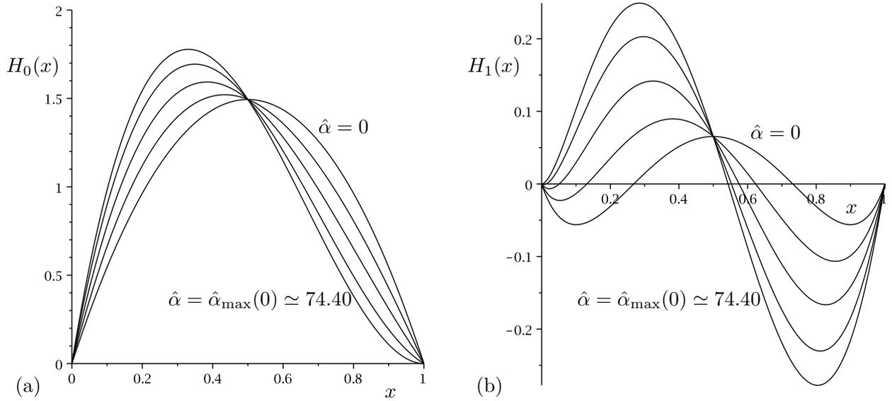
FIG. 4: Plots of (a) the leading order term,  $H_0(x)$ , and (b) the first order term,  $H_1(x)$ , in the asymptotic solution for the profile of a pinned ridge in the limit of a weak external airflow,  $\Lambda \rightarrow 0^+$ , given by (24) for  $\hat{\alpha} = 0, 20, 40, 60, \hat{\alpha}_{\max}(0) \simeq 74.40$  when  $L = 1$ .
