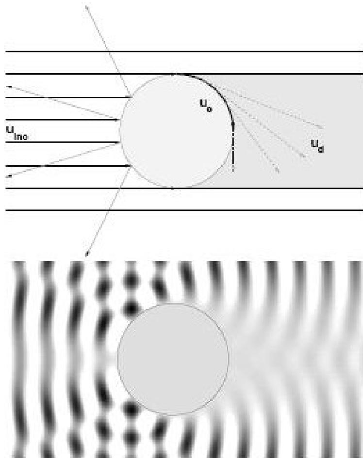
Figure 4: If obstacle is smooth then reflected and creeping rays are generated (graphic from [29]).
