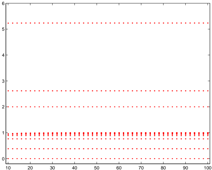
Figure: FEM calculated \text{Spec}(H, \mathbf{M}_N \times \mathbf{L}_N) plotted against N . There are no spurious eigenvalues!
