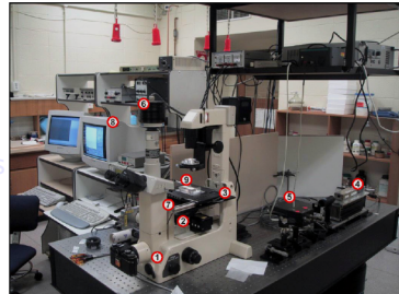
Figure 2.9: This photo was taken in June 2005, after the system was significantly modified. The components in the photo are: (1) Nikon Diaphot 300 inverted microscope, (2) Microscope objectives, (3) Microscope stage, (4) Coherent Compass 4000M Laser, (5) BEOC Laser Stabiliser, (6) MTI IFG CCD Camera, (7) Physik Instrumente Piezo Translator, (8) replacement control computer with custom written Labview software, (9) Sample Cell built in-house.
