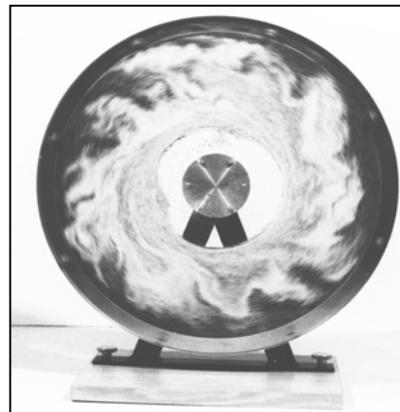
*A homogeneous dry mixture of large (dark) and small (white) particles flows in the narrow gap of a short cylindrical drum that rotates about its axis (Figs. 1 and 2). Depending upon the angular velocity of the rotation, the particles will segregate by size and form a Catherine wheel pattern (1) or they will mix chaotically (2).*
