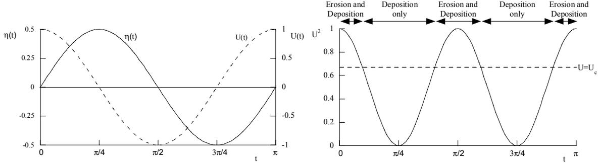
**Figure 2.** The tidal elevation  $\eta(t)$  and the velocity  $U(t)$  as functions of time. Also plotted is  $U^2(t)$ , showing the periods during which erosion and deposition occurs along with the periods with deposition only.
