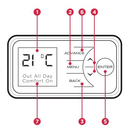
The heater is fitted with an adjustable thermostat enabling the room temperature to be controlled. The minimum room temperature is 7°C. The maximum temperature is set to 26°C by default however this can be increased to 32°C if required. A temperature of 21°C represents a normal room temperature.
